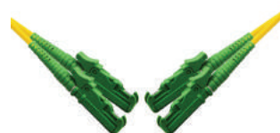
Patchcord E2000/APC-E2000/APC SM G.652D duplex 2m
